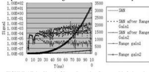
FIGURE 5 Echo Signal of Laser Detection System with Q\_laser is 1\*10-5J and t\_tx is 10ns
