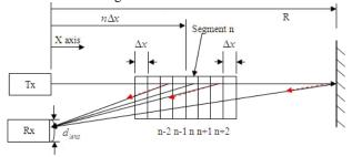
FIGURE 2 Model for the Echo Wave of the Back Scattering after the Laser Penetrating through the Non-Uniform Cloud
