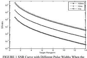
FIGURE 1 SNR Curve with Different Pulse Widths When th Extinction Coefficient of the Cloud and Mist Is 0.132
